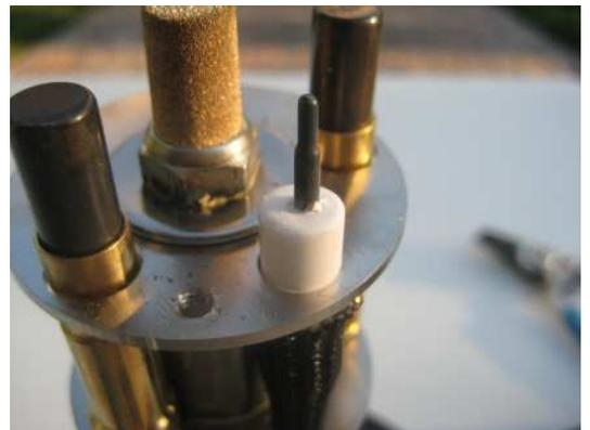
Once the Spring Clip is removed, slip the igniter out of the top washer as shown at right.
