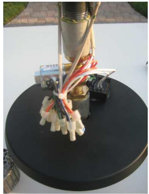
Install the new igniter by first attaching the two white wires from the igniter to the two red wires from the controller and then slip the igniter into the top washer as shown in the photo at right.
