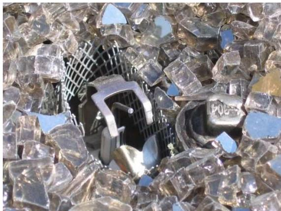
We created this fence using a galvanized steel screen material we buy in the roofing section in Home Depot. Make sure that when you install the fireglass that none of it falls inside the 'fence' you have created around the Pilot Burner. In the end, you should still be able to see the Pilot Burner as shown in this photo.
