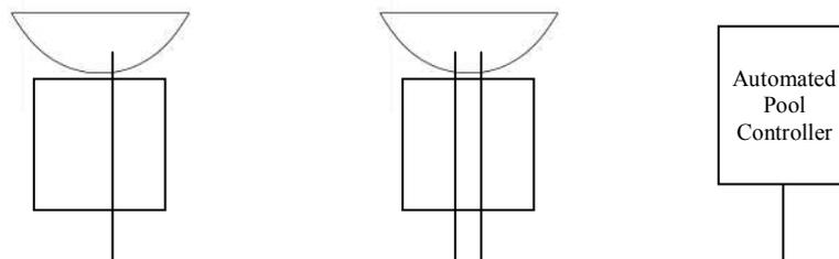
Note: In the picture at left, there is only one conduit but there are 2 pairs of wires. One pair of wires goes to the first bowl, the second pair of wires continues onto the second bowl.
